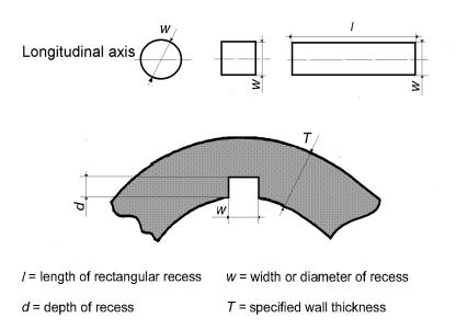
Figure 1: Reference recess forms (reference standards)
